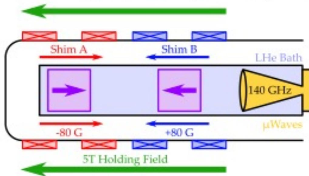
James Maxwell (JLab): Demonstration of double-sample polarization with internal shim coils
