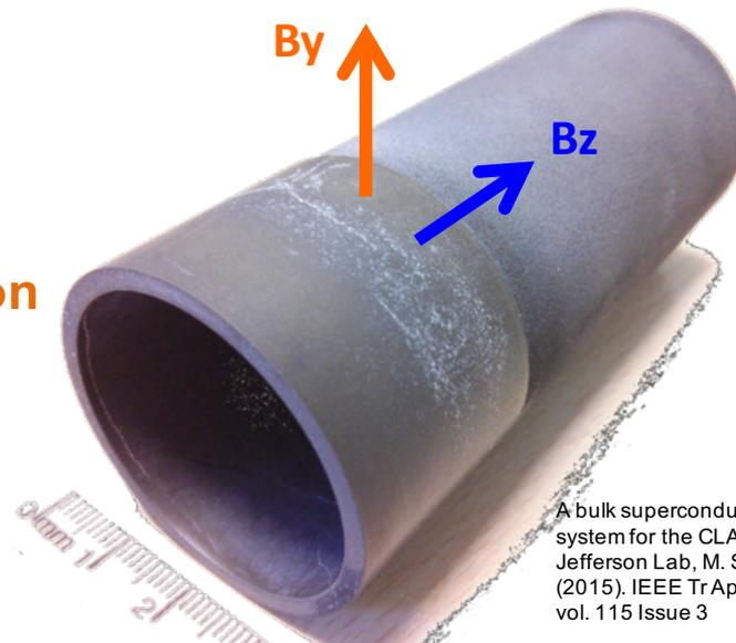
A bulk superconducting magnetic system for the CLAS12 target at Jefferson Lab, M. Statera et al. (2015). IEEE Tr Appl. Supercon., vol. 115 Issue 3
