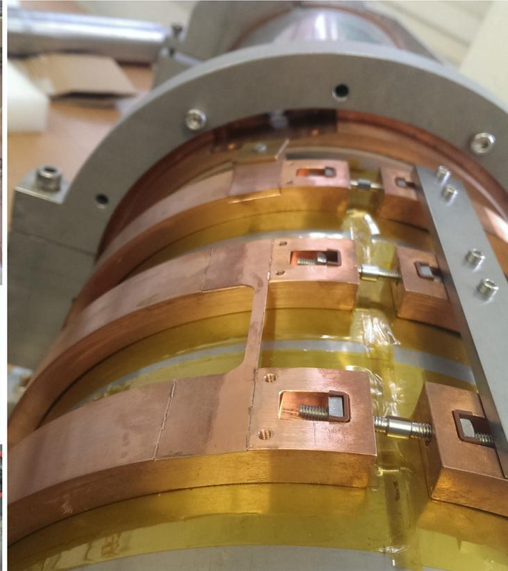
Marcel Borstein (Bonn): FEA modelling and construction of current leads for internal polarizing magnet
