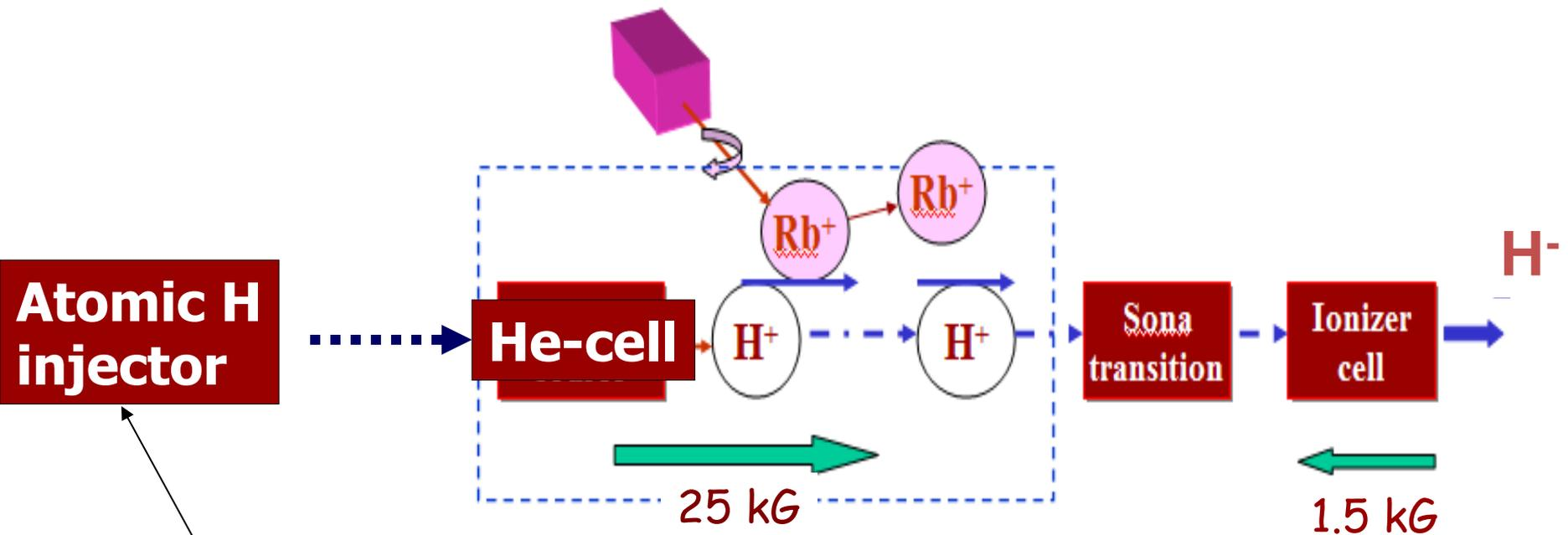
The primary proton beam and Equivalent atomic H intensity current is 2.5 A at 6.5 keV beam energy !
