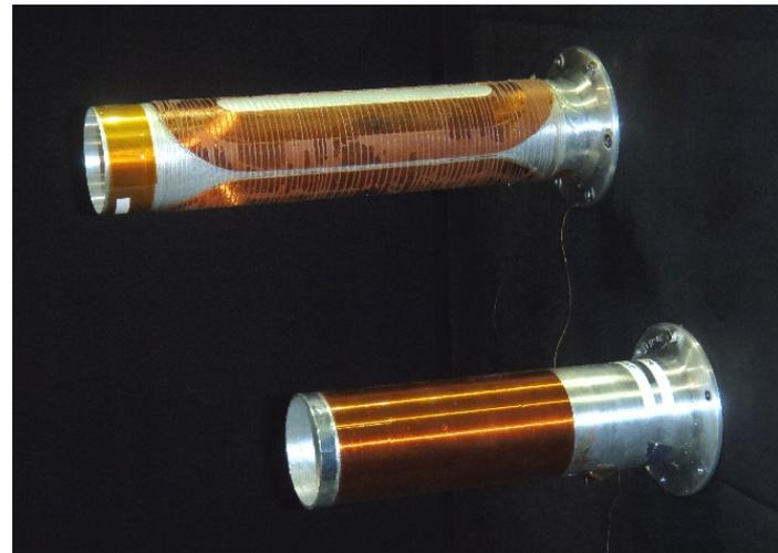
1/2 Tesla, internal holding coils
