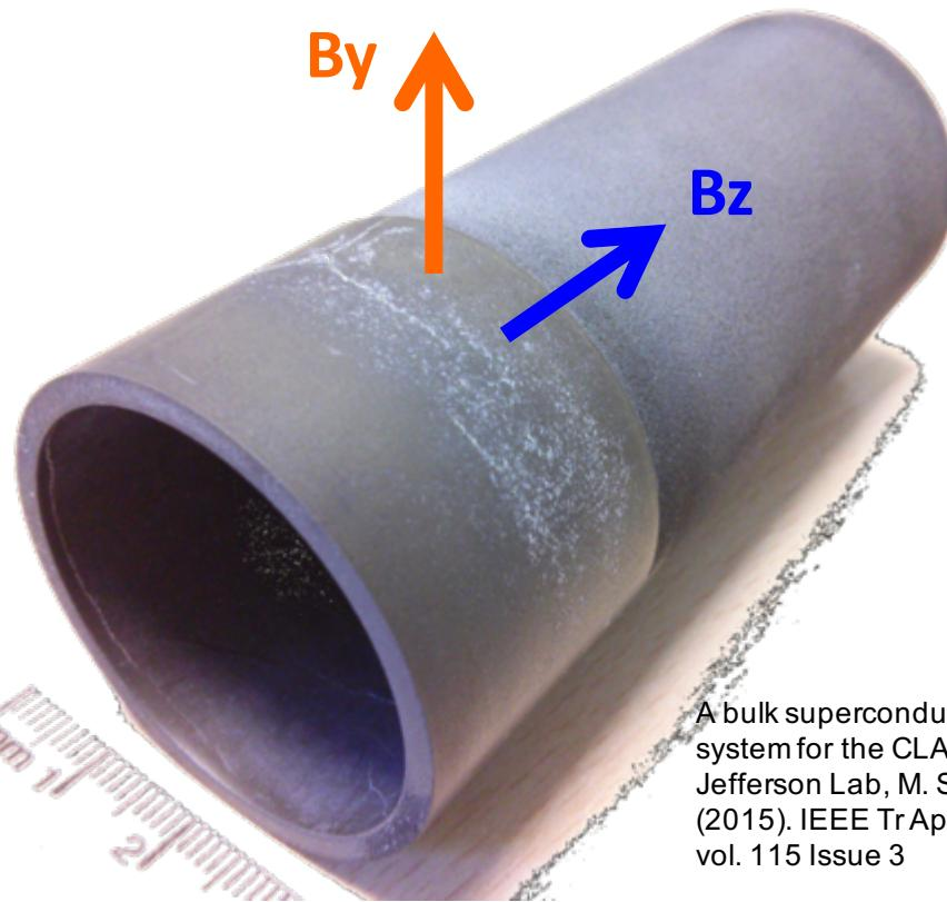
A bulk superconducting magnetic system for the CLAS12 target at Jefferson Lab, M. Statera et al. (2015). IEEE Tr Appl. Supercon., vol. 115 Issue 3
