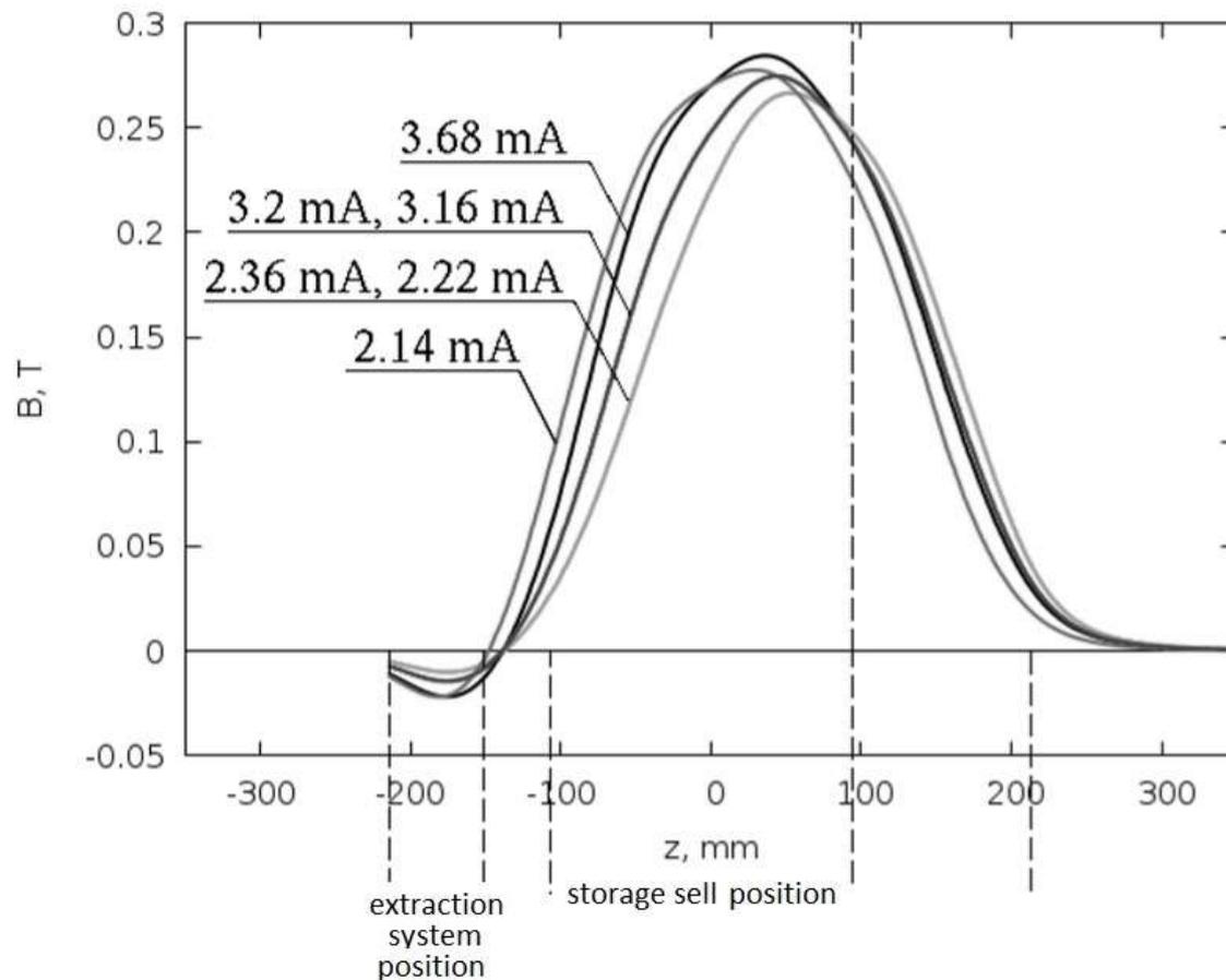
Further optimization of the magnetic field distribution in the ionizer brought the results demonstrated in Fig. At the polarized deuteron beam of 3.68 mA the unpolarized pulsed proton beam is equal to 75 mA and the beam of  $H_2^+$  ions – 3.8 mA
