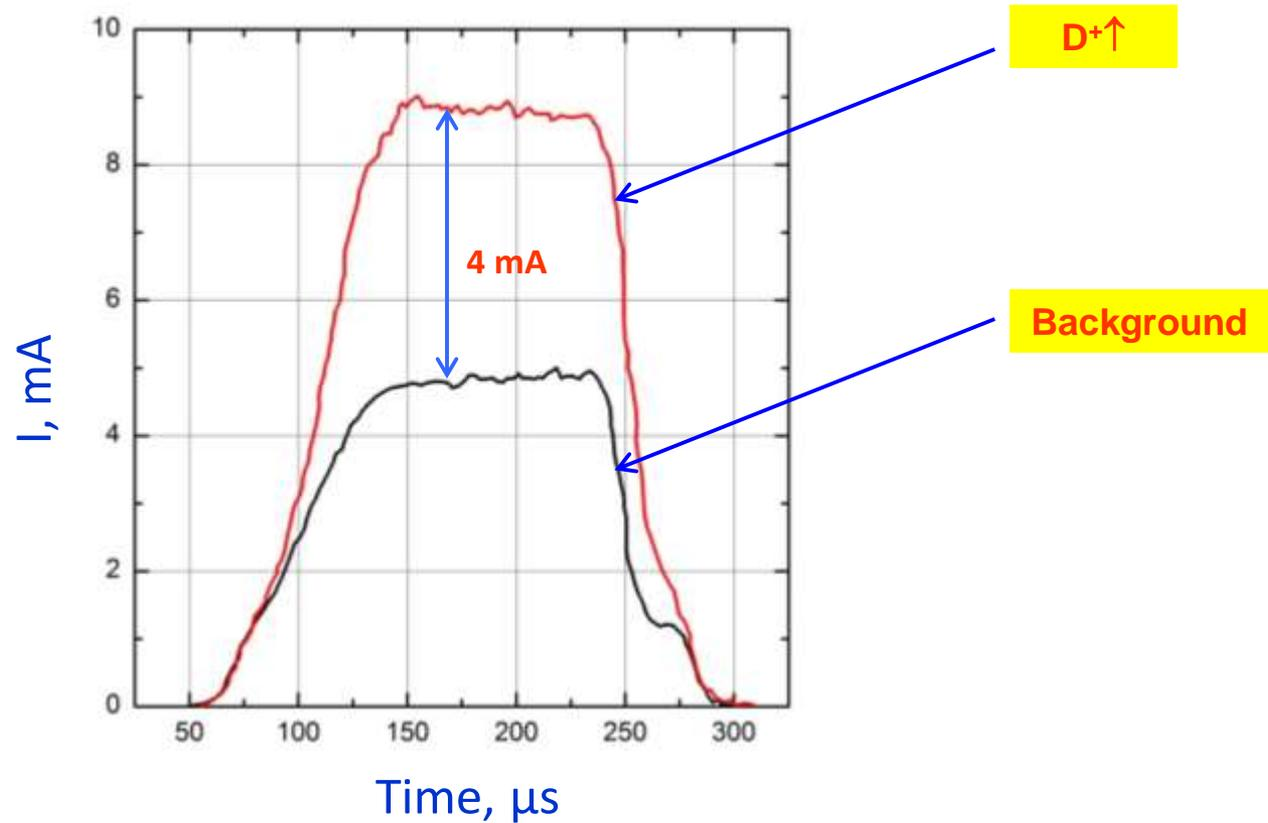
The current improvement in the SPI extraction system increased the magnitude of the polarized beam
