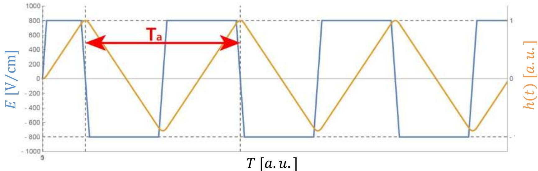
Electric field reversed every few hours, depending on  $T_2^*$  (usually  $T_a = T_2^* = 3$  h)
