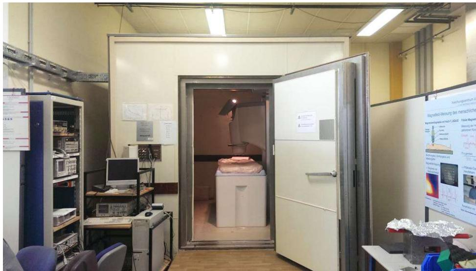
*Initial initiative to reduce the magnetic field gradients:* additional mu-metal cylinder
