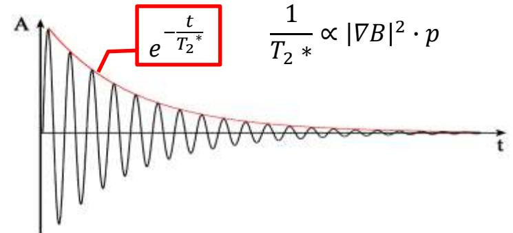
$\nabla B_{\text{res}}$  not sufficient for long coherent spin precession -  $T_2^* \sim 1 \text{ min}$
