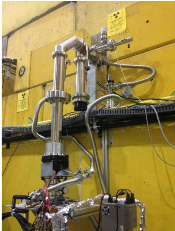
Transmission measurement of 100cm guide
