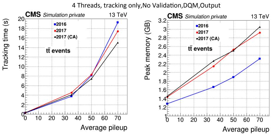
Despite an increase in seeding time, the higher accuracy of quadruplets eventually reduces combinatorics in pattern-recognition producing a significant gain in timing. No free lunch though: memory increase is sizable and action to reduce the memory footprint shall be welcome
