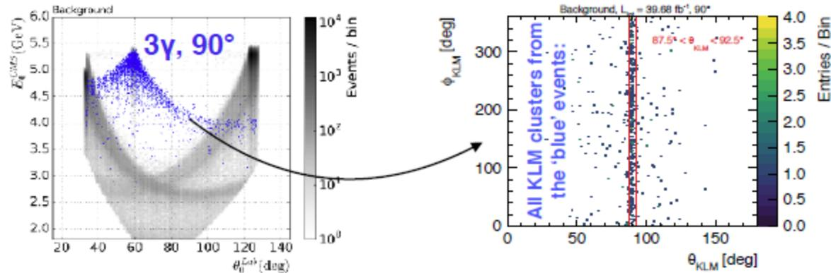
Cosmics + Phase 2  $e^+e^- \rightarrow \mu^+\mu^-\gamma$  will be used to get detailed maps of gaps and materials (cables, pipes, ...) inside the gaps
