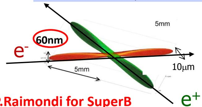
... For a 40x increase in intensity you have to make the beam as thin as a few x100 atomic layers!
