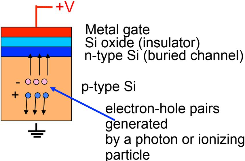
Moving charge from pixel to pixel
