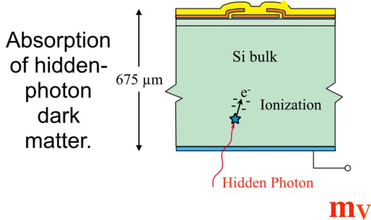
hidden photon absorption would produce  $mv / 3.6 \text{ eV}$  charge carriers in silicon:
