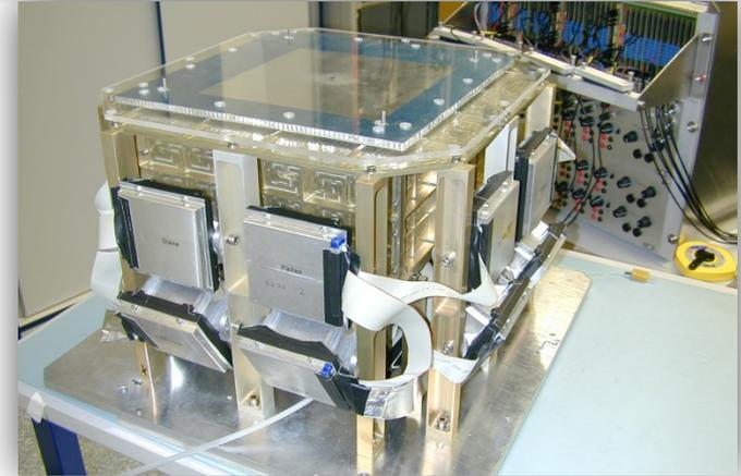
*MEGA prototype (Si-tracker & CsI Compton telescope)*
