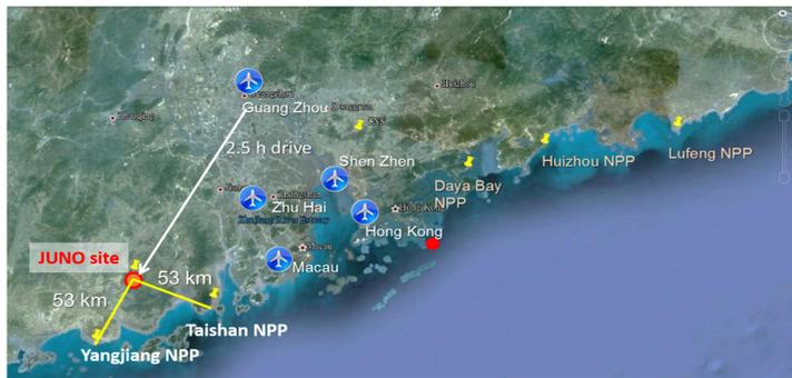
**Baseline reactors-detector about 53 km: optimized in the region of the maximum 1-2 oscillation**
