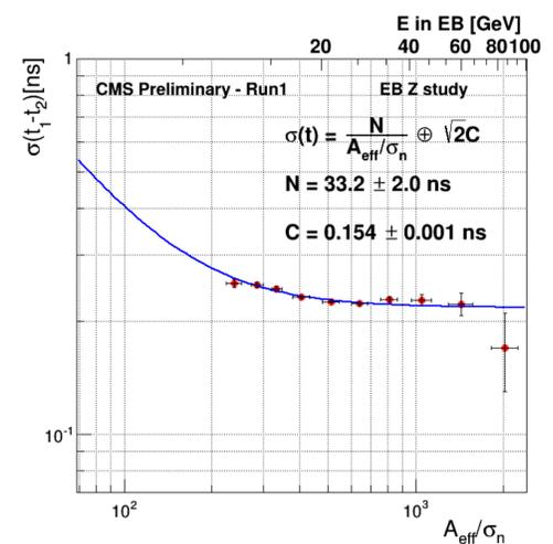
Resolution of time difference between the two electrons from  $Z \rightarrow ee$  decays, as a function of the effective amplitude, normalized to the noise in the ECAL Barrel for 2011+2012 data
