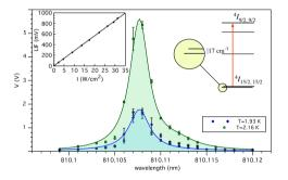
The pump laser does not affect the thermal population of the Zeeman excited level at least up to a few  $W/cm^2$  intensity
