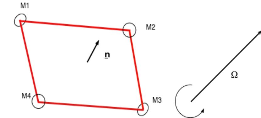
the ringlaser gyroscope is described by  $\underline{n}$  and its scale factor  $\mathbf{S}$
