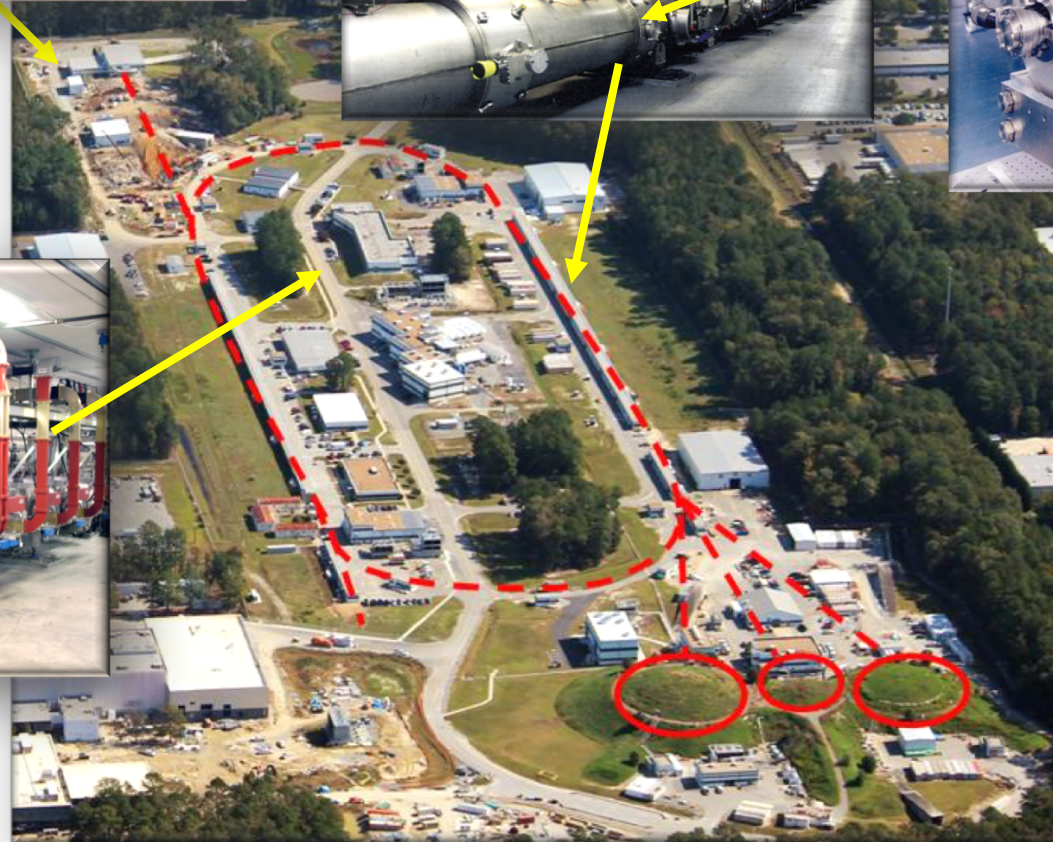
An aerial view of the recirculating linear accelerator and 4 experimental halls
