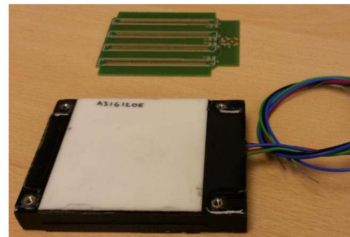
After potting, before readout PCB is attached
