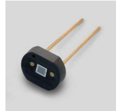
The SiPM is a matrix of diodes, each biased with a monolithic load resistance. The bias level is just above their breakdown voltage. Typically 3 V above the breakdown.
