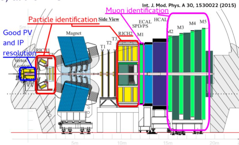
$\Delta p/p \sim 0.4\%$  at 5 GeV,  $\sigma_{IP} = 20 \mu\text{m}$  for high  $p_T$  tracks.
