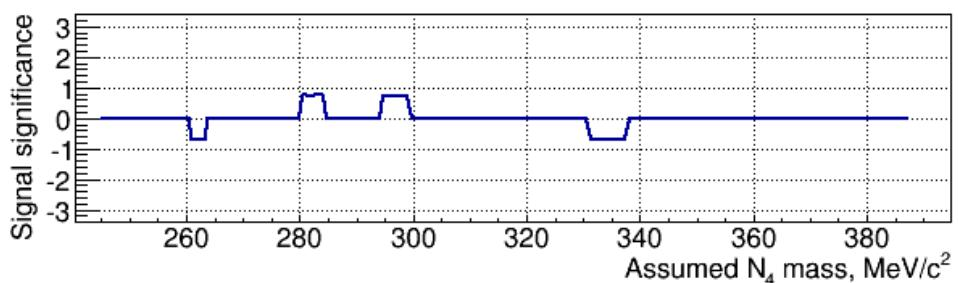
$$\text{UL}(\text{BR}(K^\pm \rightarrow \mu^\pm N_4) \text{BR}(N_4 \rightarrow \pi^\mp \mu^\pm)) = \frac{\text{UL}(N_{\text{sig}})}{N_K * \text{Acceptance}}$$
