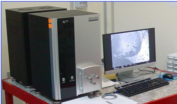
*Table-top Scanning Electron Microscope (mini-SEM) with EDS to discriminate atomic elements.*
