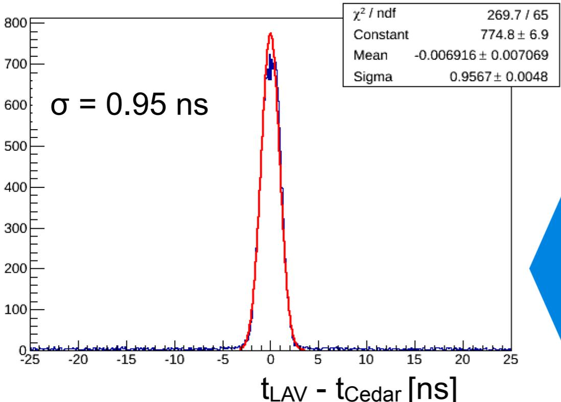
Time alignment after slewing correction
