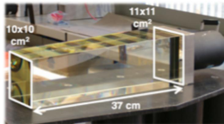
2500 crystals (Schott SF57 lead glass) with R2238 76-mm PMT  $\mu$ -metal case
