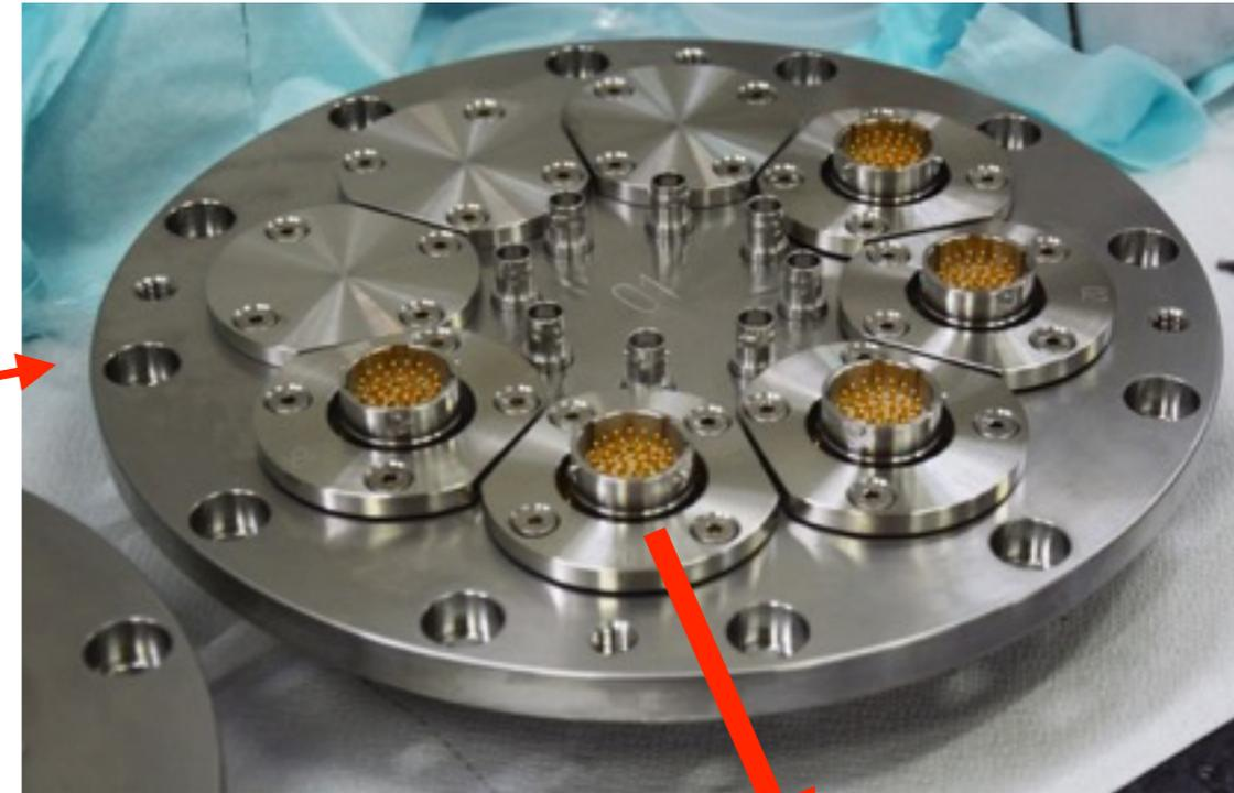
32 pin: HV supply for PMTs
