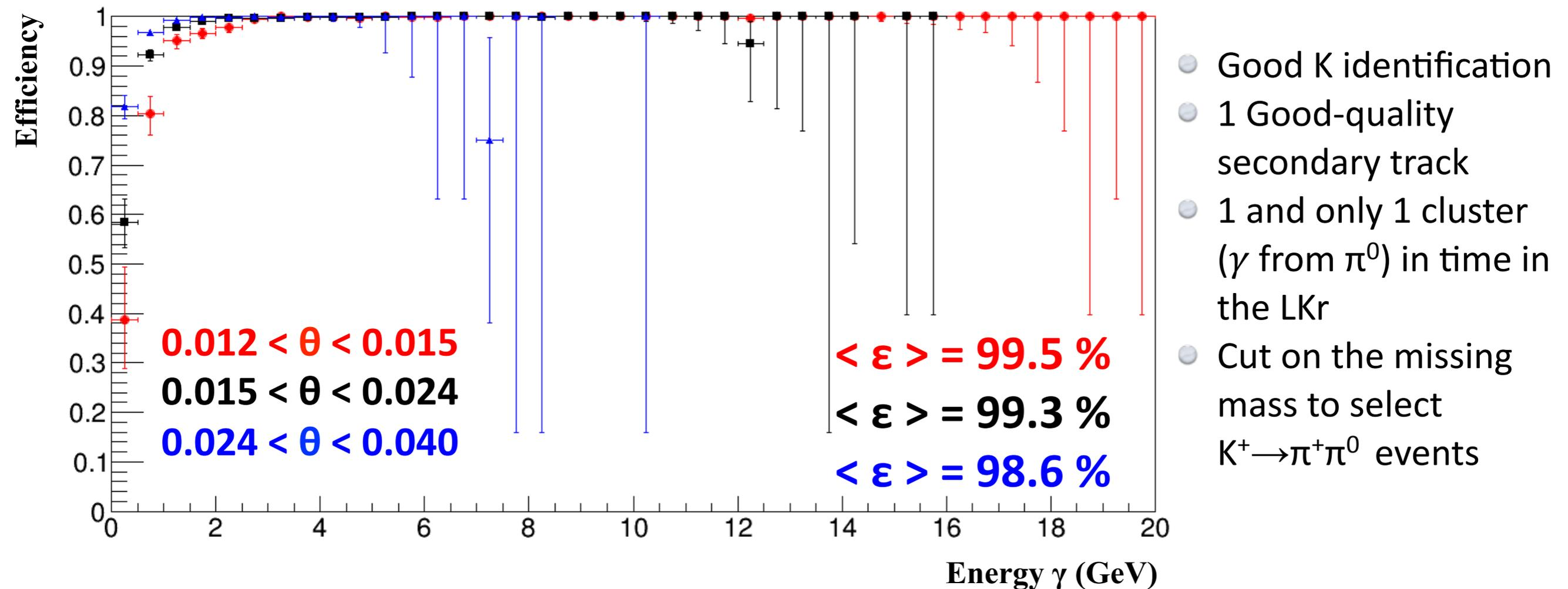
$K^+$ ,  $\pi^+$  and 1  $\gamma$  reconstructed in LKr with the 2<sup>nd</sup>  $\gamma$  expected to hit LAVs. A hit is found if at least 1 block is fired within 5 ns of the expected time.
