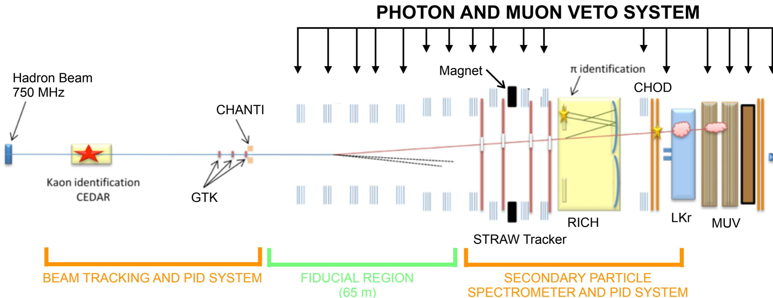
Approximately cylindrical shape around the beam axis for the main detectors.
