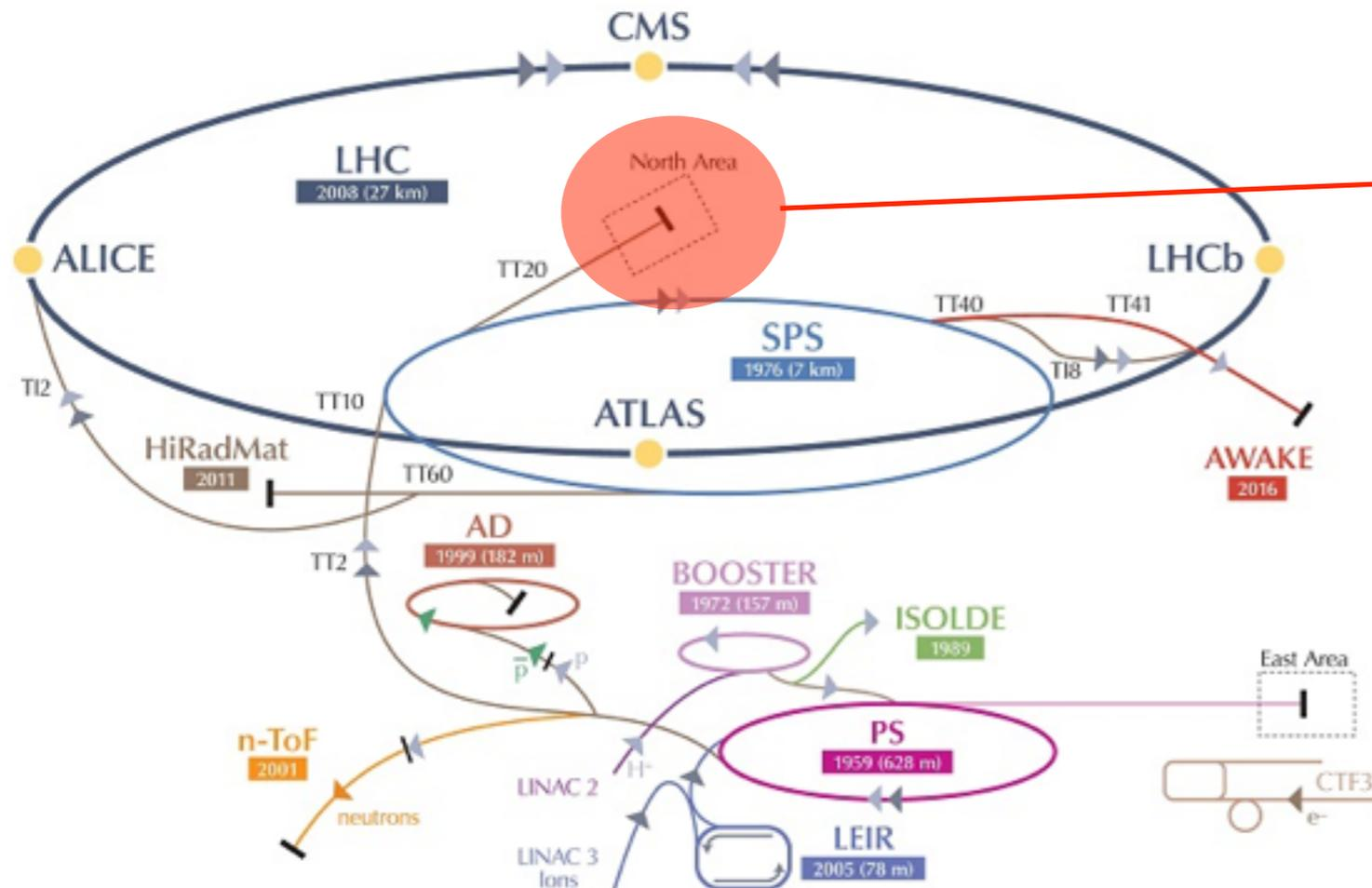
NA62 is housed in the CERN North Area. A new beam line will provide a secondary charged hadron beam 50 times more intense than in the past, with only 30% more SPS protons on target.
