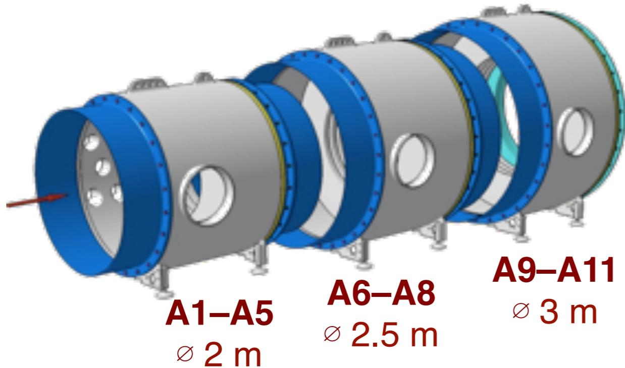
Each LAV station is made of 4 or 5 rings of lead glass crystals (from OPAL) with attached PMTs.
