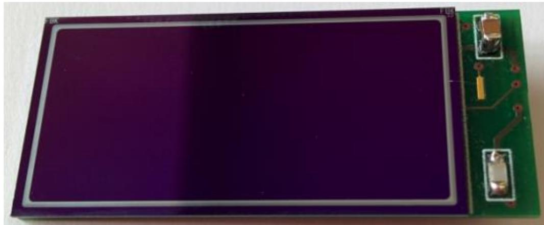
SDD-chip back side with bonding pads
