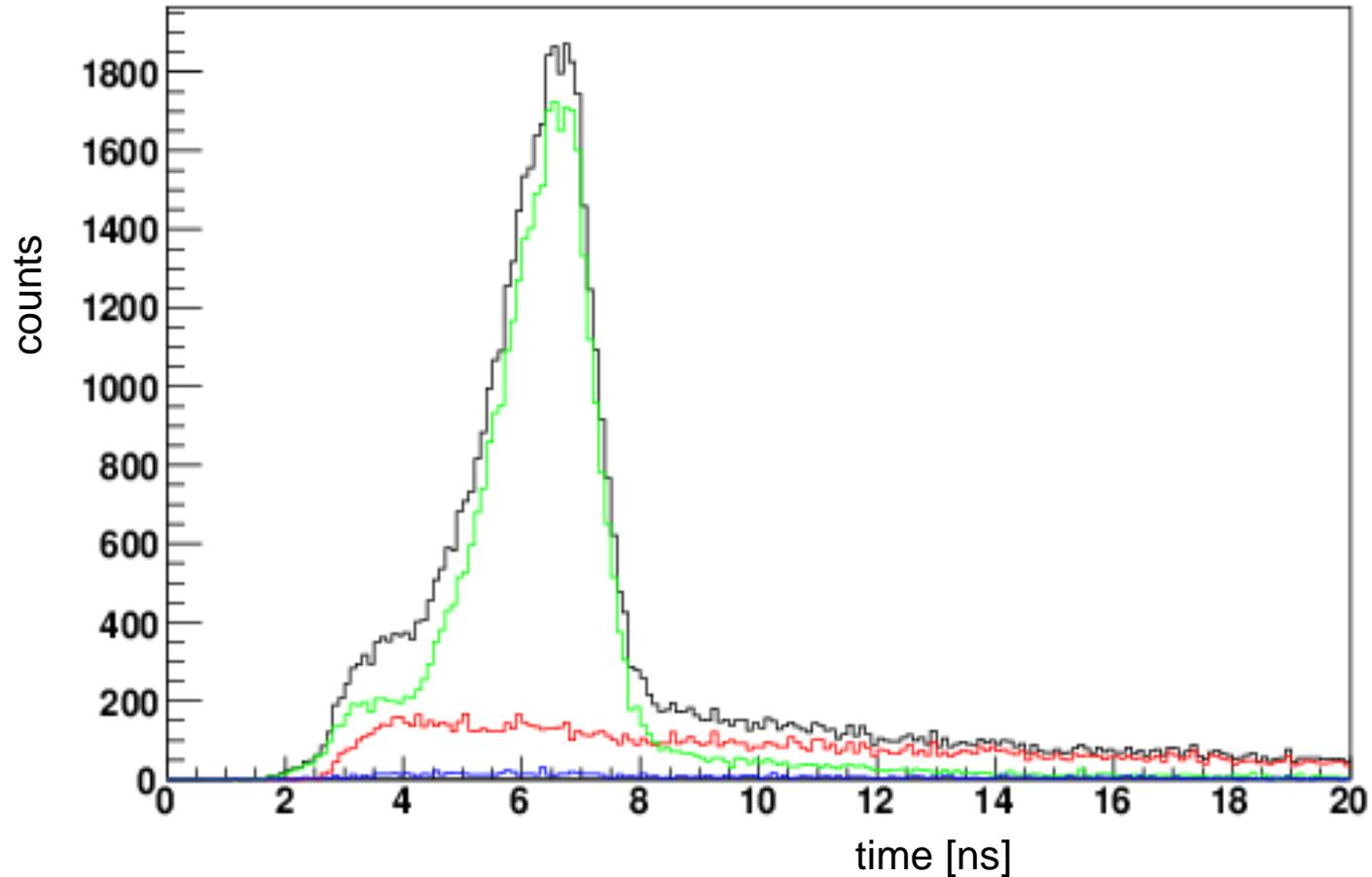
*Timing ( $< ns$ ) of veto-1 scintillators. The peak in green corresponds to particles from  $K^-$  absorption on gas nuclei. The red distribution is the time spectrum of events correlated to a  $K^+$ ; no peak is present because there is no nuclear absorption, the shape follows the  $K^+$  decay. In blue, the bottom kaon detector detects neither a  $K^+$  nor a  $K^-$ .*
