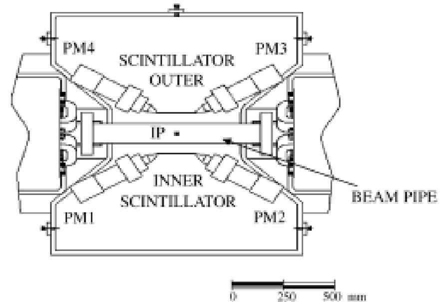
Fig. 1. The Kaon Monitor experimental setup in the DEAR region at the DAΦNE interaction point (IP).
