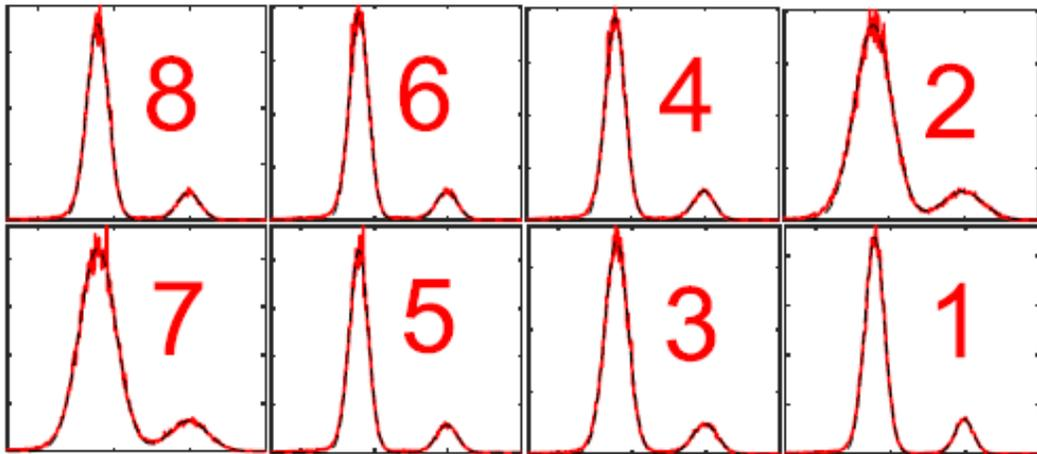
Fig. 5. Eight X-ray spectra acquired by irradiating a 2x4 SDD array with an un-collimated  $^{55}\text{Fe}$  X-ray source at a temperature of  $-30\text{ }^{\circ}\text{C}$  with  $3\text{ }\mu\text{s}$  shaping time using.
