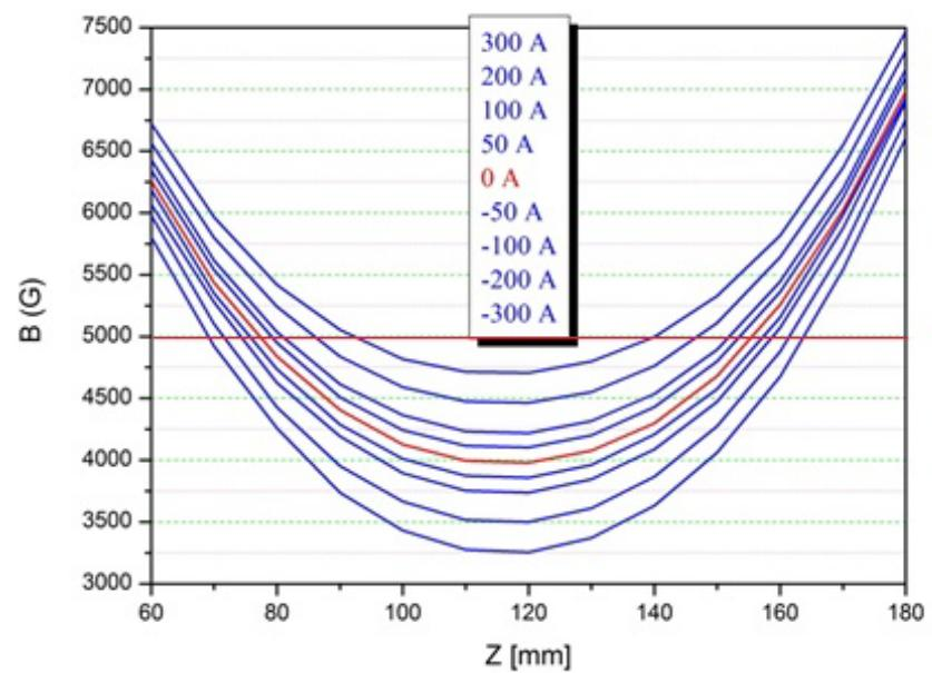
Adjustment of  $B_{\min} \pm 750$  G
