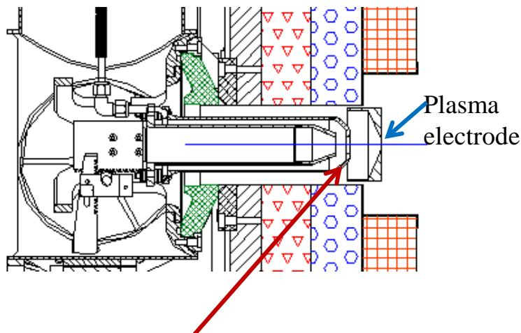
Puller electrode- negatively biased and water cooled
