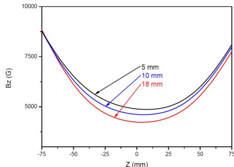
Correction of  $B_{min}$  with soft iron plates
