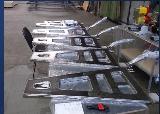
Blocks of azimuthal trimming coils (GKMP, Bryansk, Russia)
