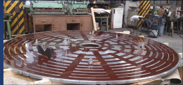
Block of radial trimming coils (EVPU, Slovakia)
