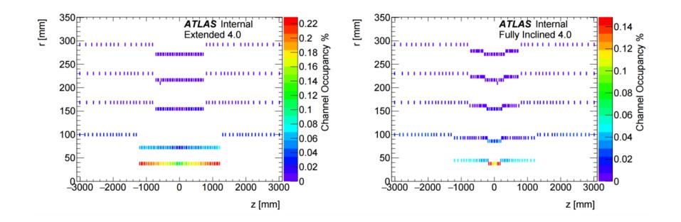
Pixel occupancies for a minimum bias event with a pile up of 200 Channel occupancy higher in extended (as expected)
