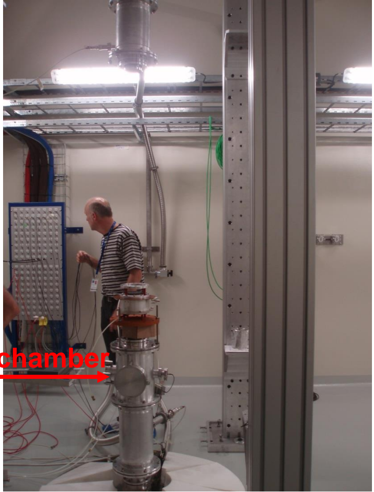
SiMon2 detector removed with its flange and replaced with the Silicon Telescope Setup.
