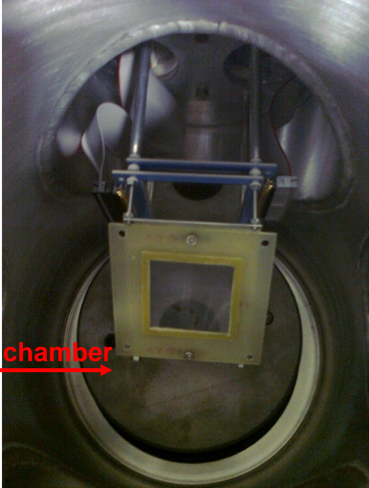
SiMon2 detector removed with its flange and replaced with the Silicon Telescope Setup.
