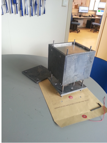
Figure 3: The scattering chamber built for the measurement.
