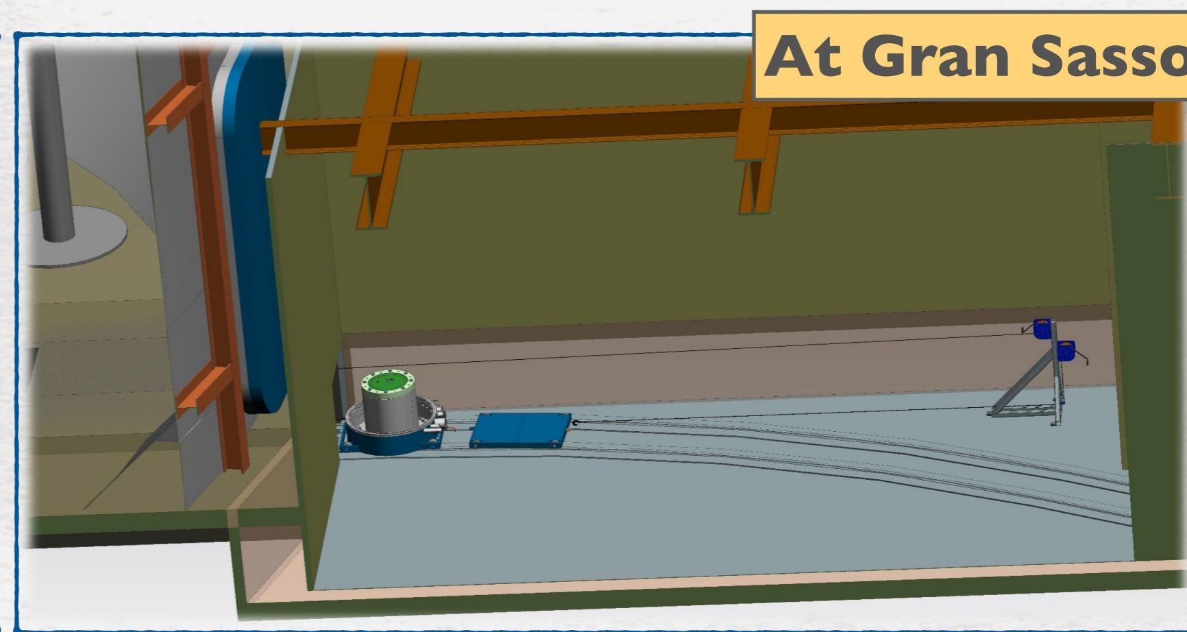
The **activity** is obtained by measuring the **heat released inside the shield and absorbed by a water flow**
