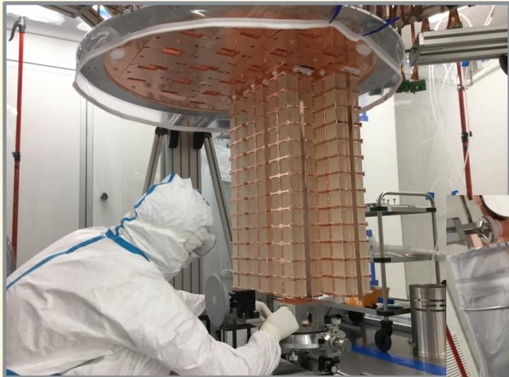
Detector “protective bag” flushed with nitrogen during installation stops
