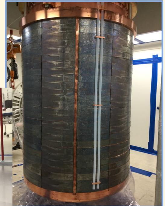
8 tons of internal Pb shielding
