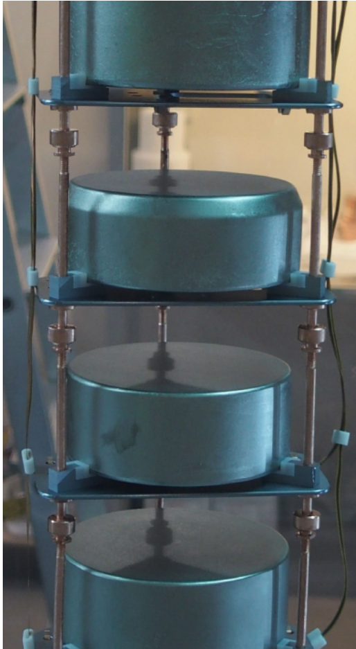
New low-mass detector holder (silicon, copper, PTFE)
