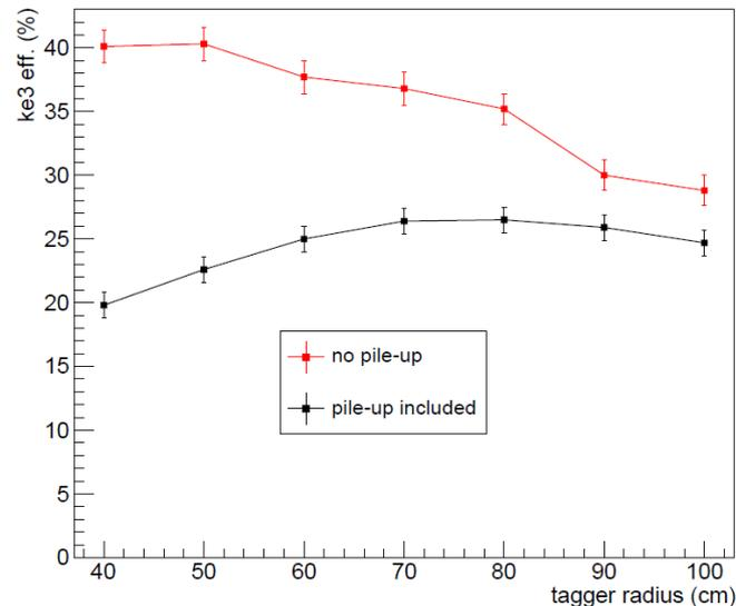
Pile-up effect on Ke3 efficiency seen at nominal rates. Mitigation enlarging the radius: ~ 25 % (~ 50 % purity).
