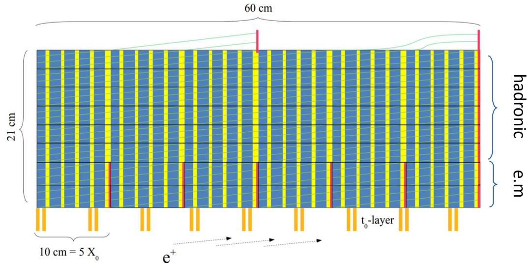
**(1)** Compact shashlik calorimeter (UCM) with longitudinal ( $4 X_0$ ) segmentation.
