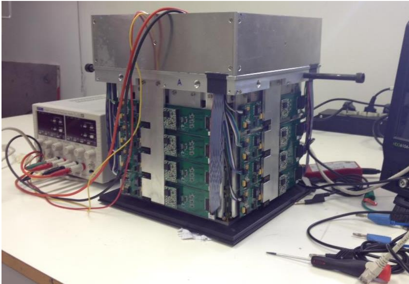
Assembled dose profiler @ INFN Roma - SBAI Courtesy of G. Traini, V. Patera and G. Battistoni
