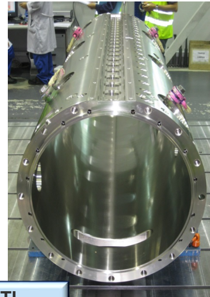
First DTL girder
