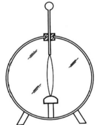
Fig. 6. Schematic view of the Wulf electrometer.
