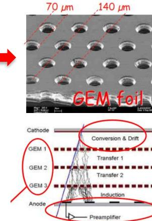
Up to **MHz/mm<sup>2</sup>** of primary electrons for  $^{20}\text{Ne}$  30 MeV/u on  $\text{C}_4\text{H}_{10}$  20 mbar
