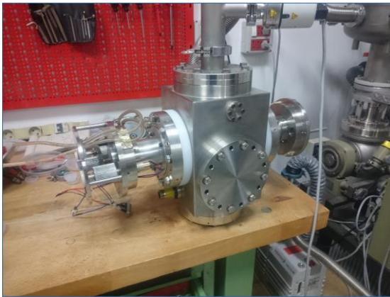
Low emittance beam line for test of tracking detectors
