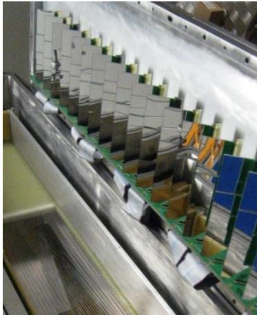
To wall of **2500 SiC-SiC pad telescopes**
