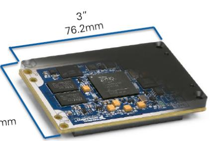
The image shows a NI System on Module (SOM) board. It is a rectangular module with a blue PCB and various electronic components. A callout box indicates its dimensions: 3" (76.2mm) by 2" (50.8mm).
