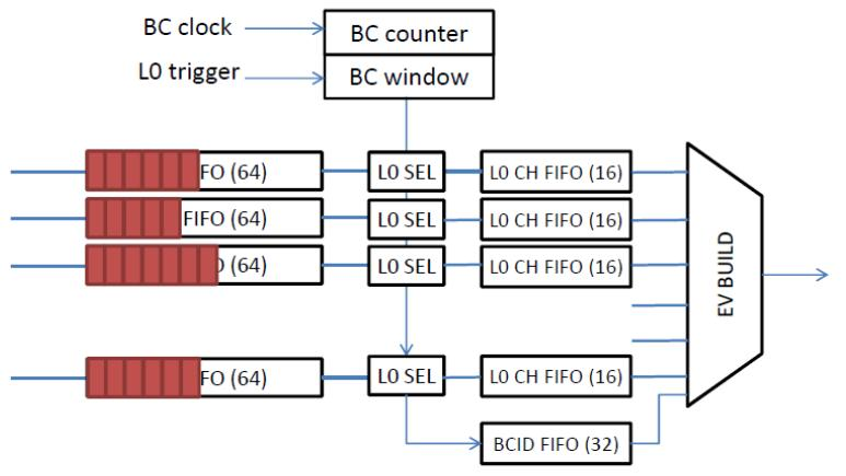
**Latency FIFO takes data from the mixed-signal front-end**
