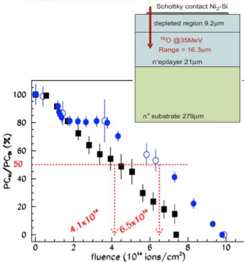
Ratio of peak centroid of  $^{16}\text{O}$  energy spectrum
