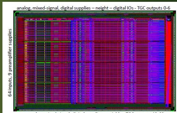
130nm 1.2V 8-metal CMOS technology from IBM
