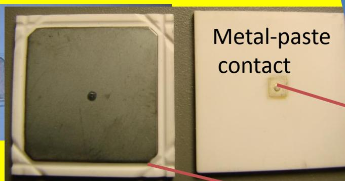
$\text{Al}_2\text{O}_3$  250  $\mu\text{m}$  spacers
