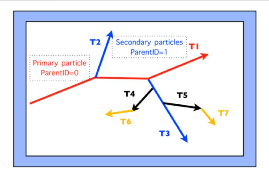
Secondary saved at the top of the stack: tracking order follows **'last in first out'** rule: T1  $\rightarrow$  T3  $\rightarrow$  T5  $\rightarrow$  T7  $\rightarrow$  T4  $\rightarrow$  T6  $\rightarrow$  T2
