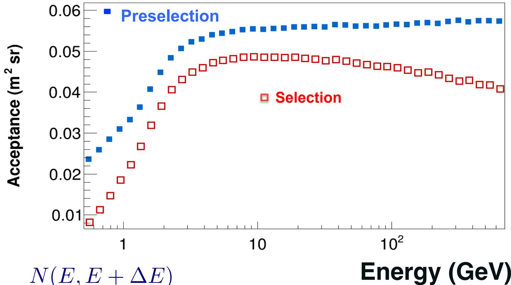
$$\Phi(E) = \frac{N(E, E + \Delta E)}{\Delta E \Delta T_{\text{exp}} A_{\text{eff}} \varepsilon_{\text{trig}}}$$
