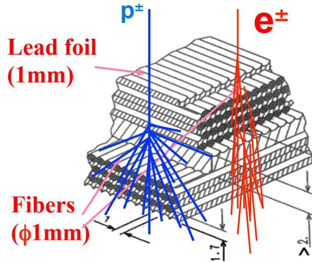
50,000 fibers,  $\phi = 1\text{ mm}$
