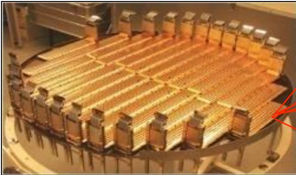
Electromagnetic Calorimeter (ECAL)
