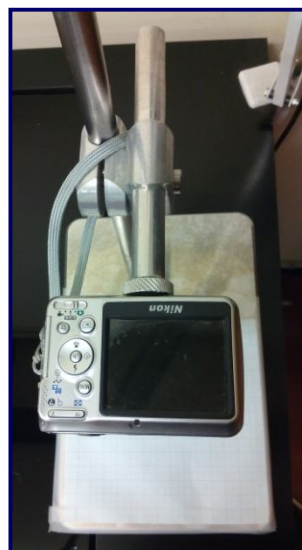
System based on the software ImageJ for the thickness measure- ments of films produced by rolling
