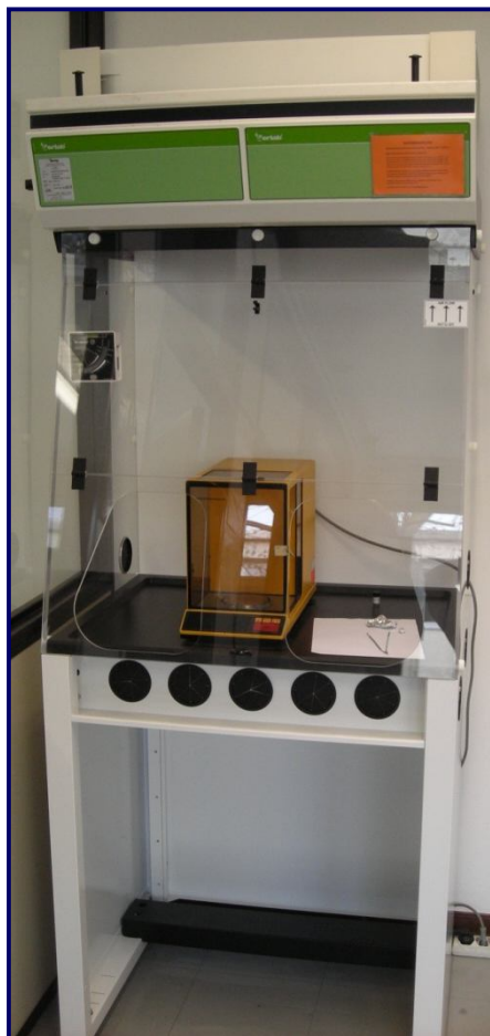
Equipment for weighing dusts (Fume hood + precision balance)
