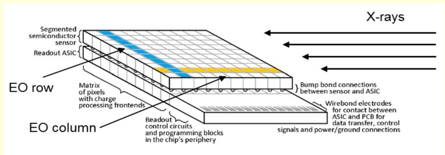
Schematic of the detector edge-on (EO) illuminated. Usually the detector is used in face-on, with the X-rays coming from above, perpendicularly to the detector matrix. Here the detector is rotated by 90°, with the X-rays impinging on the side of the sensor.
