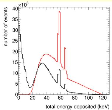
On the left, in red the energy spectrum of the source, in black the detected energy spectrum are plotted. The difference between the two is due to the limited volume of the detector and the way the X-rays interact with it.
