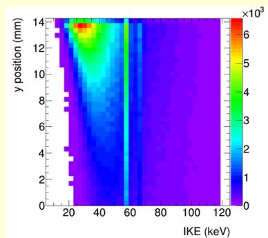
On the right, number of interactions as a function of the depth in the detector (y = 14.08 mm corresponds to the EO row 255 and y = 0 mm to the EO row 0) and of the Initial Energy of the incoming photon. The energy of the interacting photons increases with decreasing the EO row.
