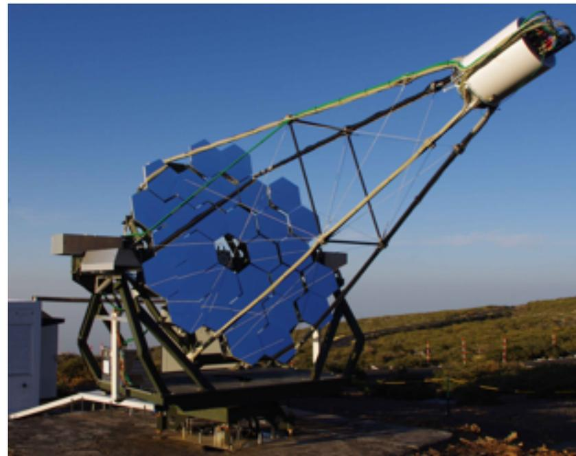
**New approach, use fully digital SiPM-based camera on a Davies-Cotton telescope.**
