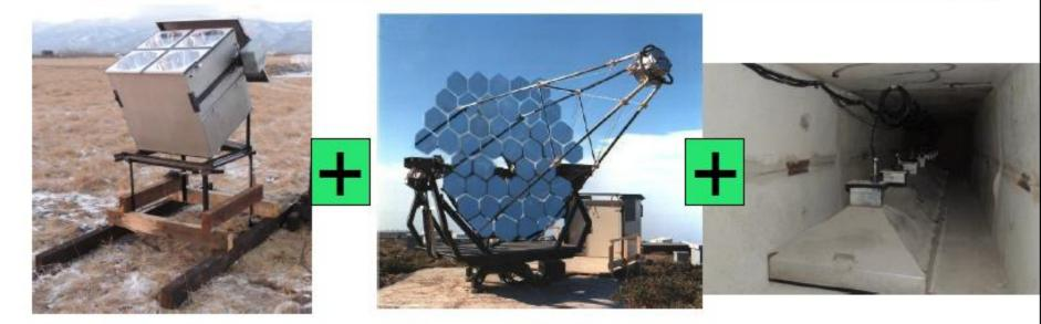
• 500 wide angle optical station on the 5 km<sup>2</sup> area, energy threshold 30 TeV
