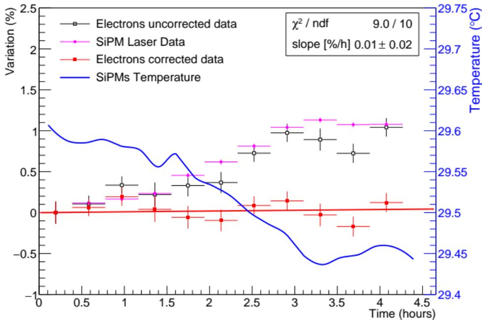
$$\text{Electron corrected data} = \frac{\text{Electron uncorrected data}}{\text{SiPM laser data/Monitor data}}$$
