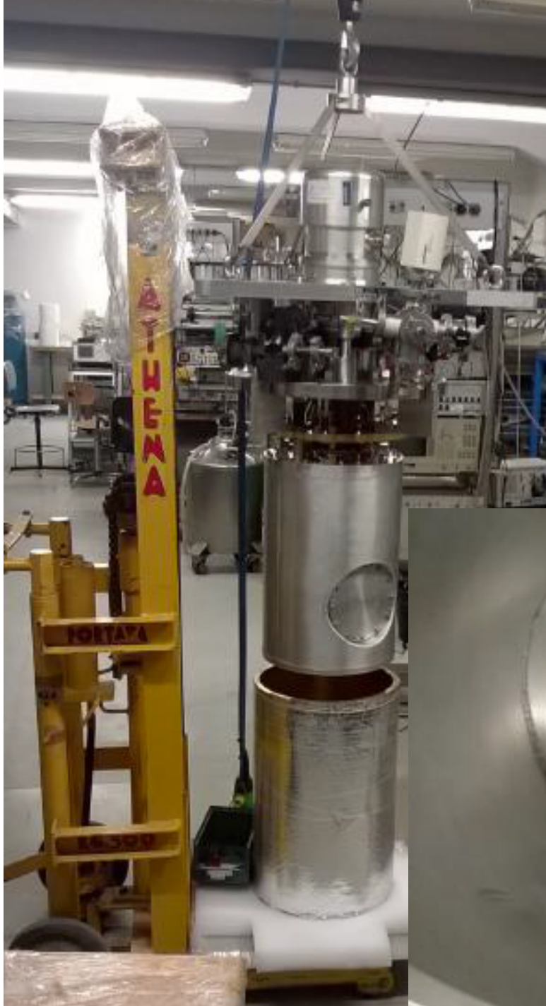
Cryogenic optical lever at 1550 nm using InGas PSD
