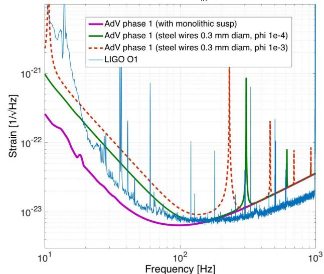
Inspiral range (Mpc), steel wires on 4 TM,  $\phi$  = 1e-4 (1e-3)
