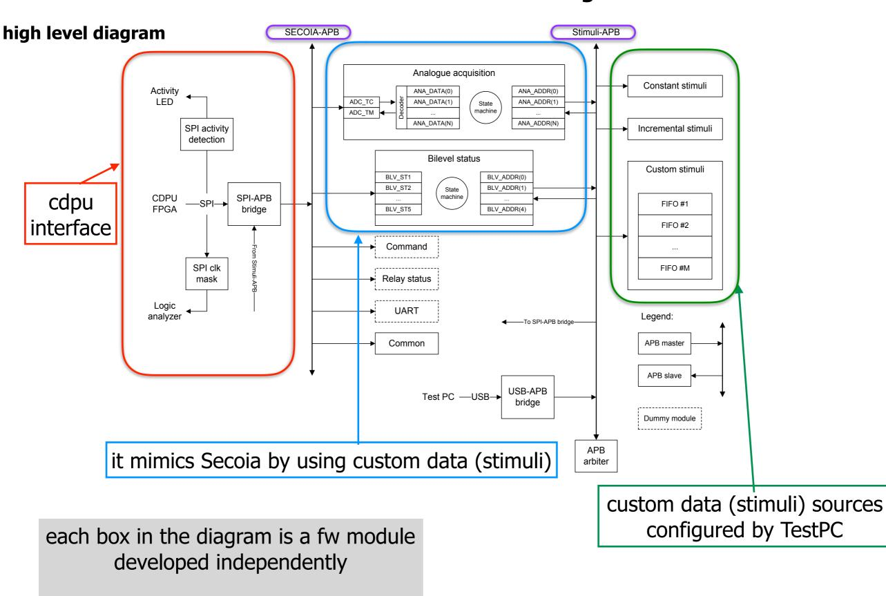
Modules are connected using APB bus
