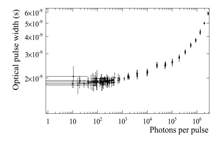
Generally good performance, pulse widths of <3ns at 100,000 photons/pulse
