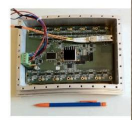
Size: 1/10 of a T2K TPC FEC, for the same number of channels. Flat readout achieved for a pad size of  $3x7 \text{ mm}^{**}2$ . We plan to use a pad size  $\sim\sim100 \text{ mm}^{*}2$
