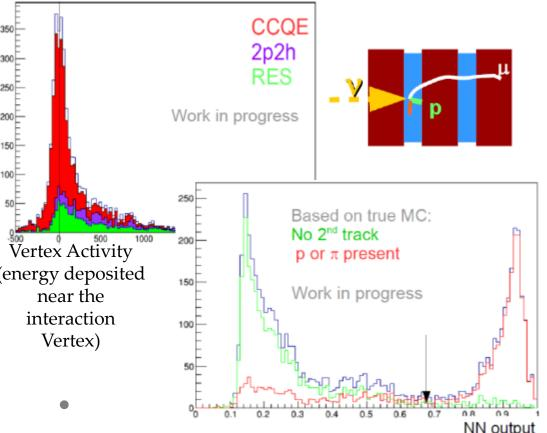
•For selected events with reconstructed 2 tracks (μ and *p*) an additional short track has been searched using set of vertex activity variables given to a **neural network**
