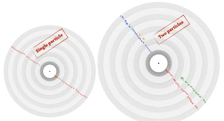
The new CDC track finder is able to identify tracks on cosmic rays events with an efficiency close to 100% (i.e. each triggered event contains at least one track). A few interesting events with more than one particles are also correctly reconstructed. All the CDC hits are represented.
