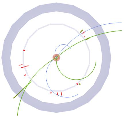
(b) A correctly reconstructed tag-side  $B^- \to D^{*0} e^- \bar{\nu}_e$  decay (with  $D^{*0} \to D^0 \pi^0$  and  $D^0 \to K^- \pi^+$ ). A low-energetic final-state-radiation photon from the  $D^0$  decay was missed.
