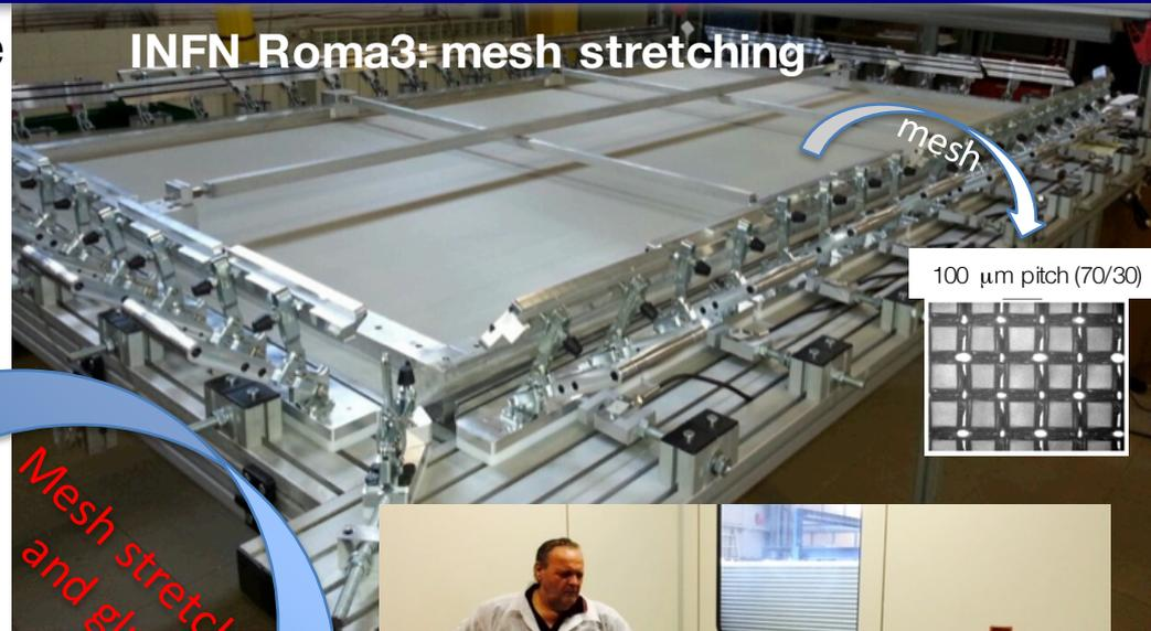
Mesh stretching and gluing
