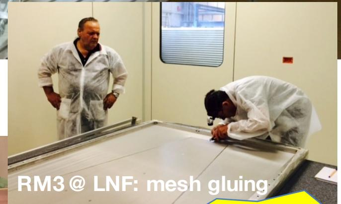
The drift panels must be “dressed” (completed) with a pre-stretched mesh
